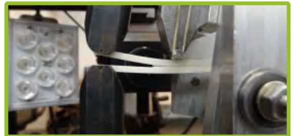
Mixed-Mode-Bending experimental test.
